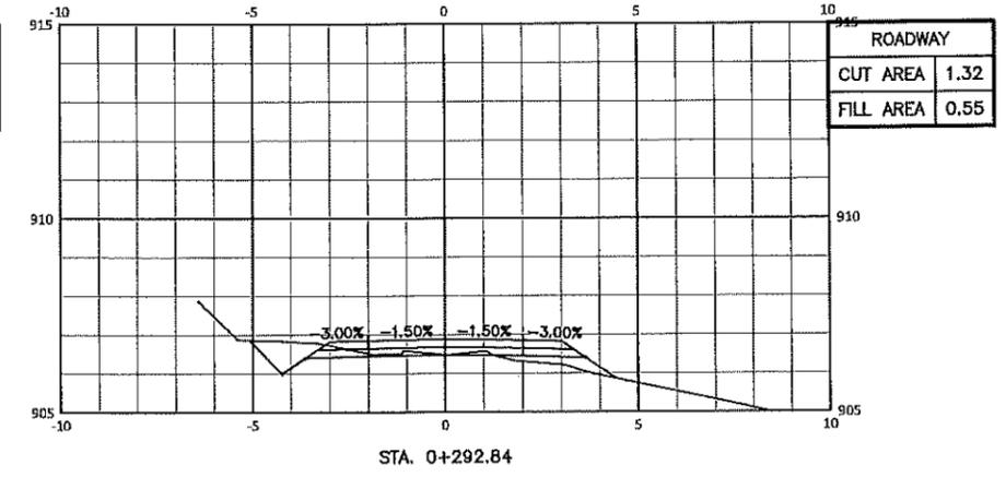
**CROSS SECTION (SECTION A)**
