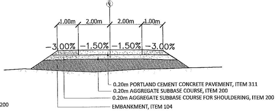
TYPICAL THRU CUT AND FILL SECTION
